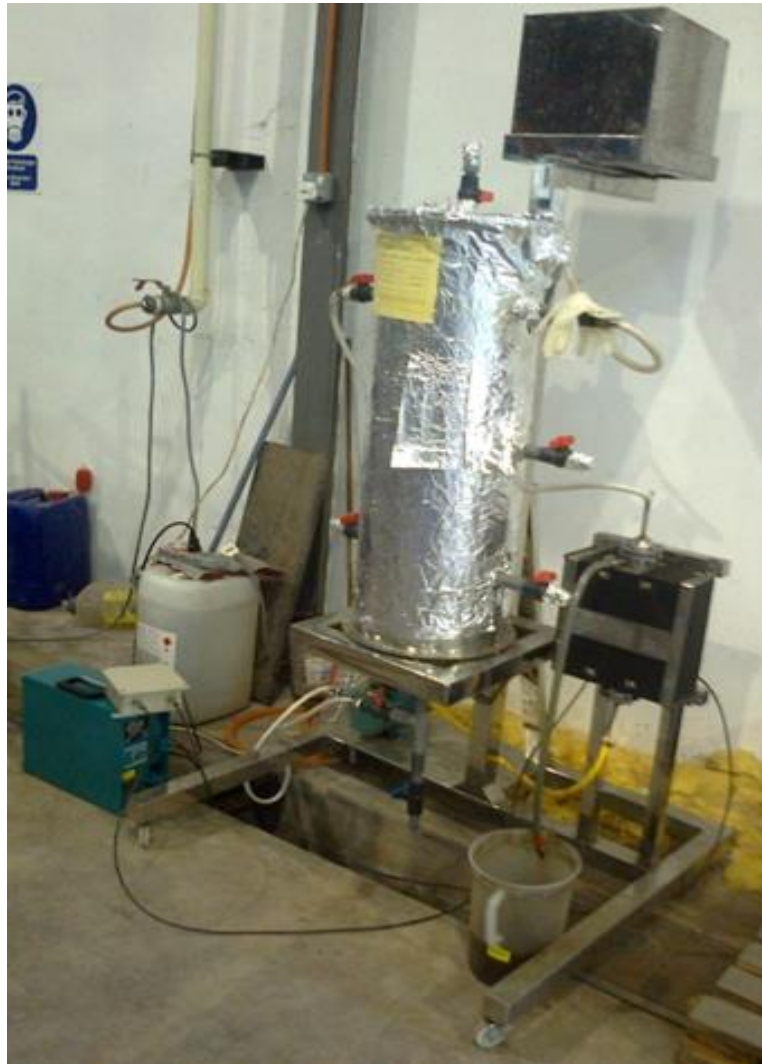
Figure 3.2: Ultrasonicated membrane anaerobic system.
