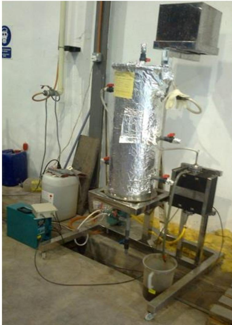
**Figure 3.2:** Ultrasonicated membrane anaerobic system.
