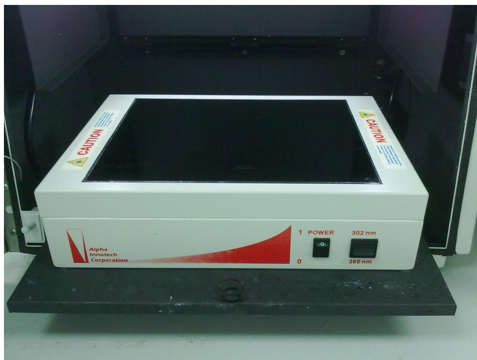
Figure C-12: The wavelength of UV used is 302 nm
