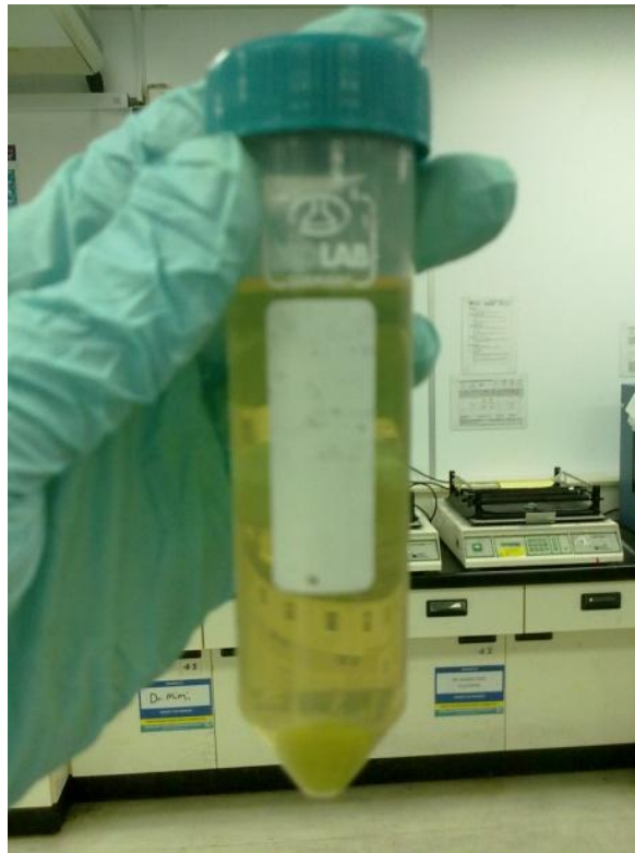
Figure C-3: The light green cell pellet (EGFP) inside the supernatant after centrifugation
