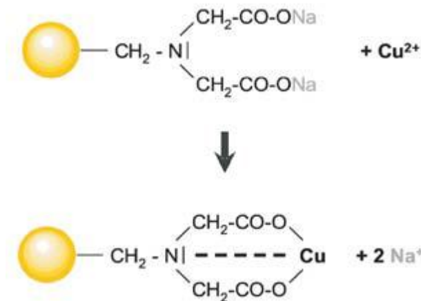
Figure 2.12: Mechanism of Binding of Copper ion to the Functional
