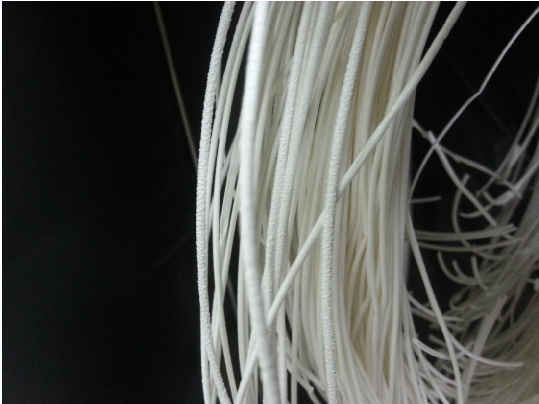
Figure 4.1: Surface of the Membrane for 10wt% PVP dope solution
