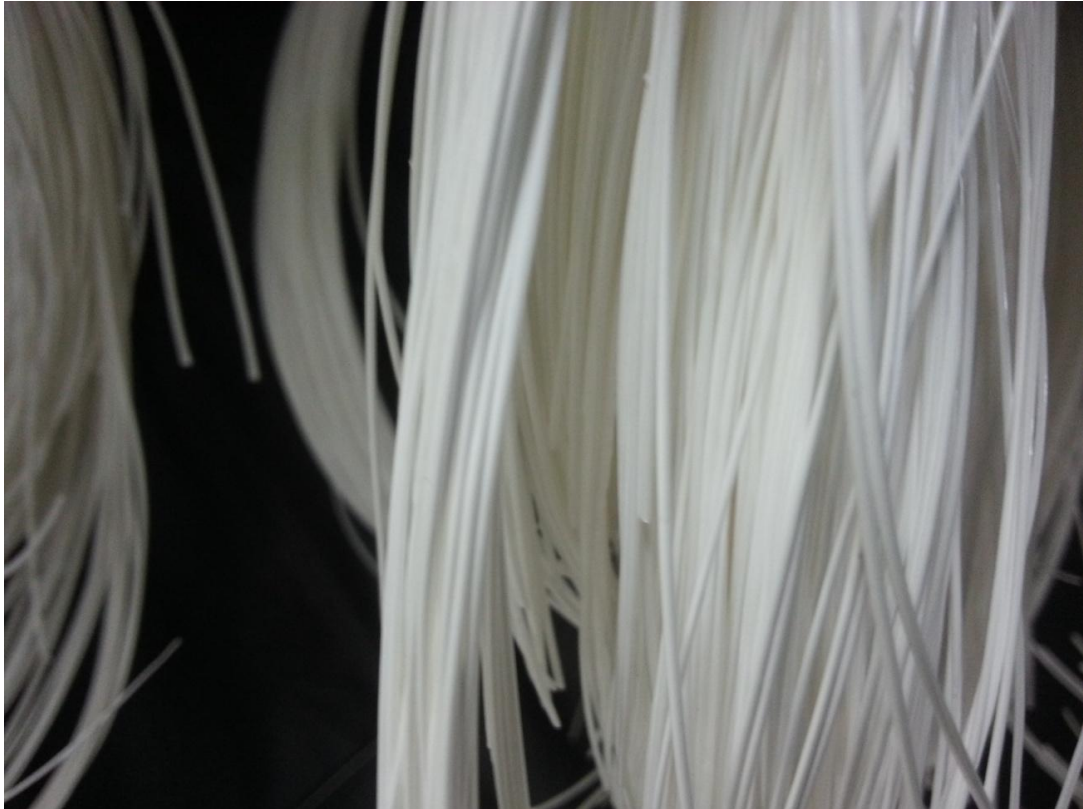
Figure 4.2: Surface of the Membrane for 0wt% PVP dope solution
