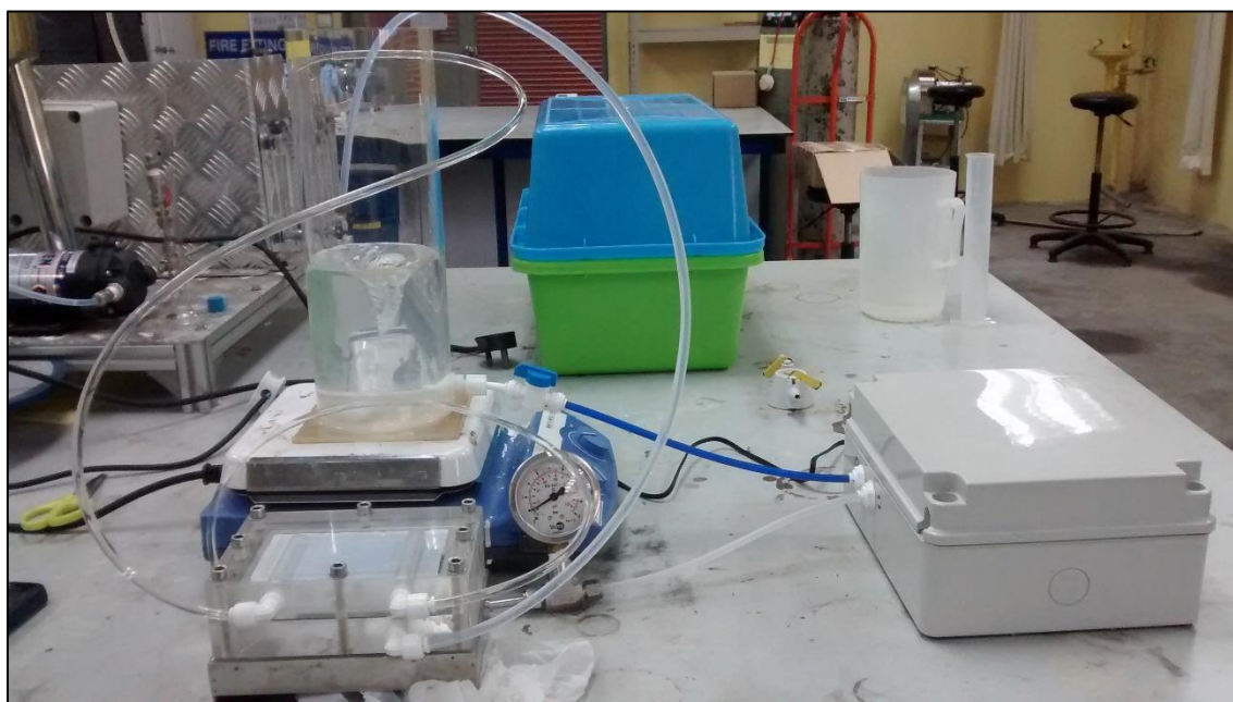
Figure 3-12: Cross flow machine.
