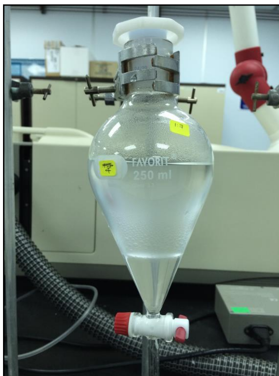
Figure 3.6: Extraction using separatory funnel
