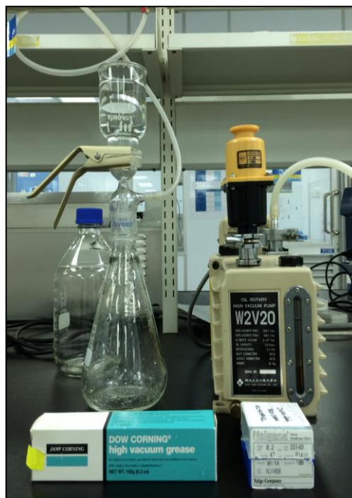
Figure 3.11 : Mobile Phase preparation (Vacuum filtration)
