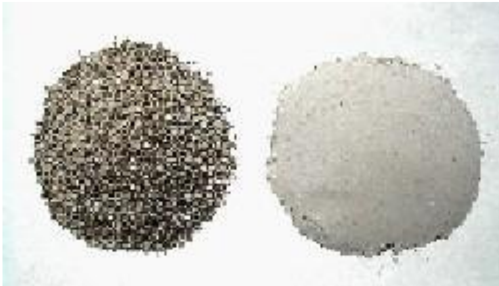
Figure 9 LCD Screen Powder After Crushed by Plastic Crusher
