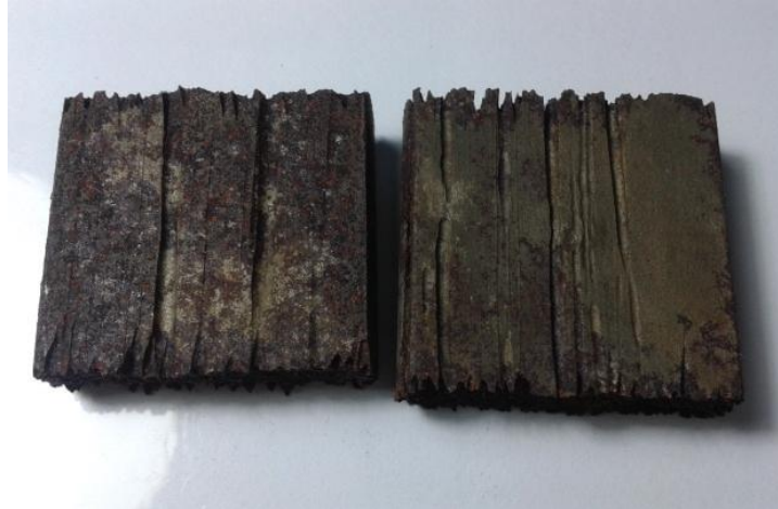
Figure 3.8: Corroded steel coupons after 7 days of the experiment.
