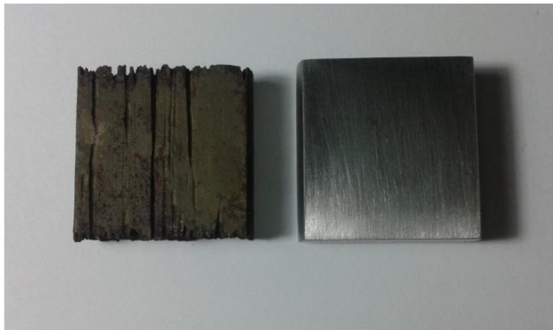
Figure 3.3: Difference between corroded and clean steel coupon.
