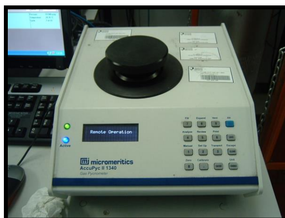
Figure 3.6: Micromeritics AccuPyc II 1340 Gas Pycnometer
