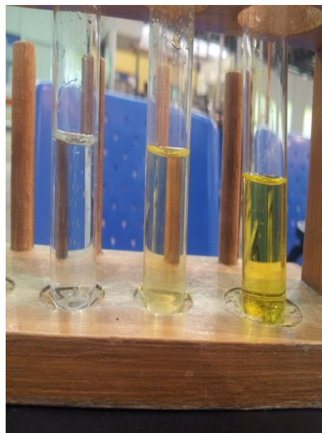
Figure 4-3 The pure methanol, the sample and the Jones oxidation reagent after diluted with water to run in UV-Vis spectrometer
