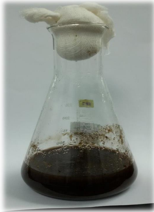
Figure 3.4: Fermentation process in Erlenmeyer shake flask with mixture of BSW and co-culture.
