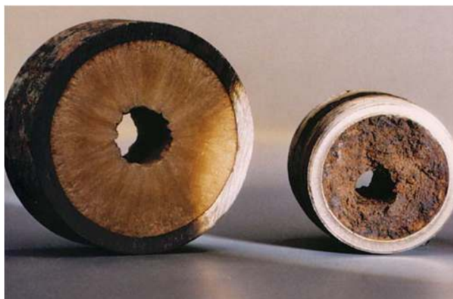
Figure 2-3: Scale in tubing (Sandengen, 2006)
