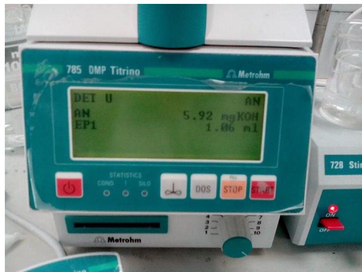
Figure 20 The acid value result was appeared on the screen of Potentiometer Titrator after reaction was completed
