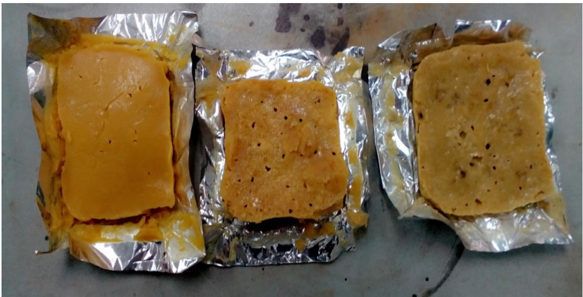
Figure 22 The polyurethane form after 24 hours
