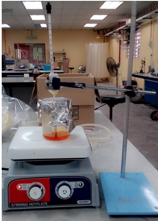
Figure 16 Process of synthesis EPO to polyol
