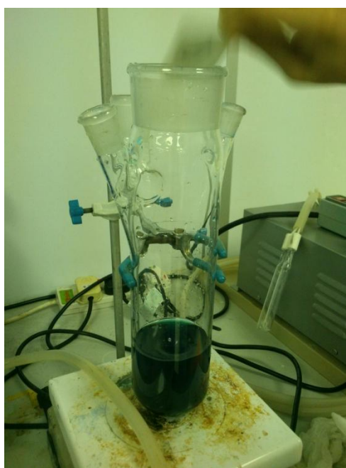
Figure 3-9: Addition of catalyst into the larger diameter housing of photoreactor containing methylene blue solution.
