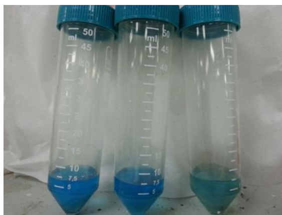
Figure 4-8: Phtocatalytic effect on methylene blue (increasing time from left to right).
