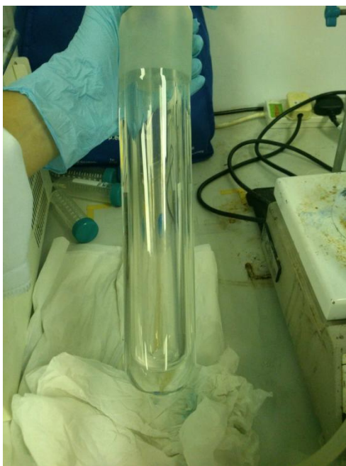
Figure 3-8: Xenon lamp housing of photoreactor.
