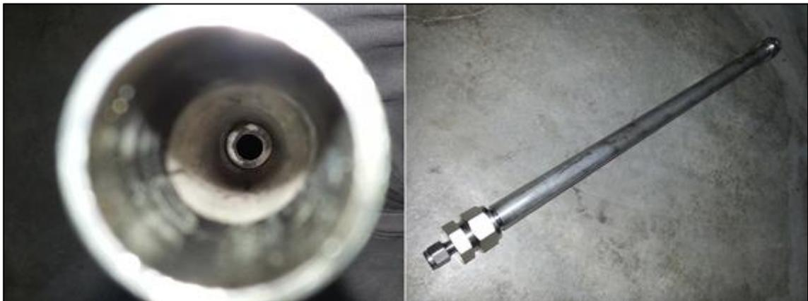
Figure 3-3: Stainless steel reactor and its support ring
