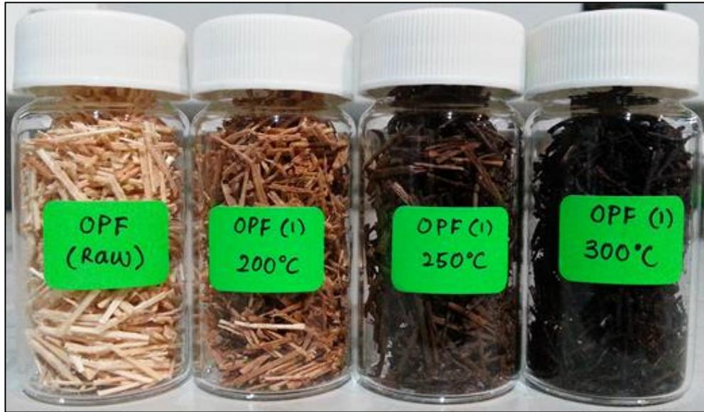
Figure 4-1: Raw and torrefied OPF samples
