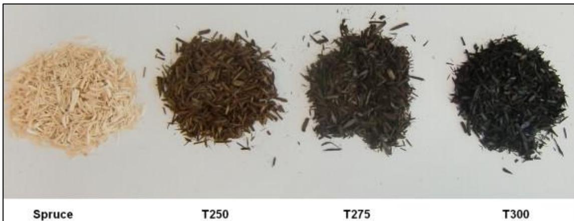
Figure 2-12: Colour change during torrefaction process (Stelte *et al.*, 2011)
