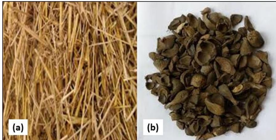
Figure 2-13: Colour of lignocellulosic material (a) Soft: rice straw (b) Hard: palm kernel shell (PKS)
