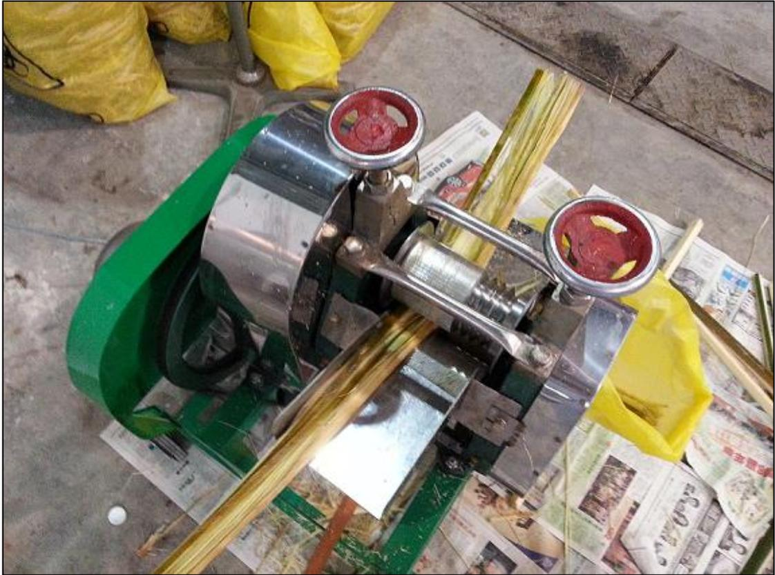
Figure 3-1: OPF fibres produced from press machine
