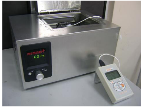
Fig. 2. Thermal Conductivity measurement setup using thermal constant analyzer technique
