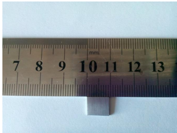
Figure 1: Sample of P11 steel
