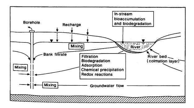
Figure 2.2: Riverbank filtration (RBF) process
