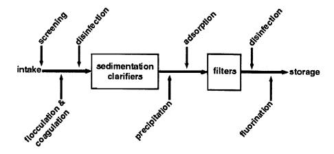
Figure 2.1: Conventional Water Treatment Process
