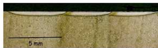
Figure 2.4: Optical micrograph showing overlap (M. A. Montealegre)
