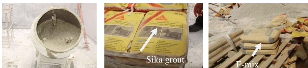
Figure 2.20: Example of grout material either used placement or pumped method
