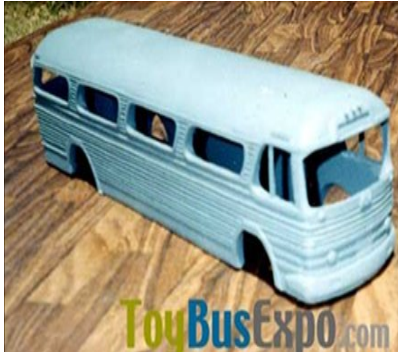
Figure 2.6: Slush Casting Product
