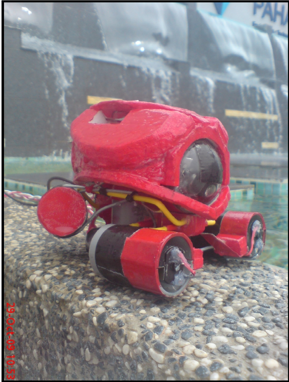
Figure 6.9: Finished prototype with attached weight
