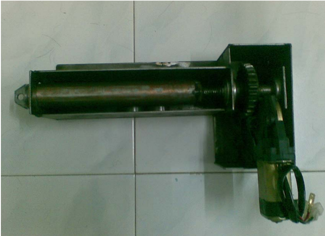
Figure 4.27: Fabricated automatic gate mechanism
