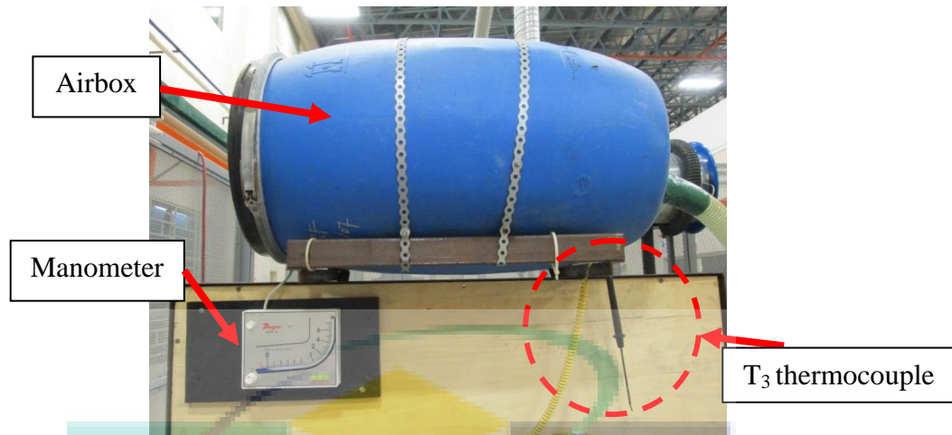
Figure 3.41: Thermocouple placement for ambient temperature measuring
