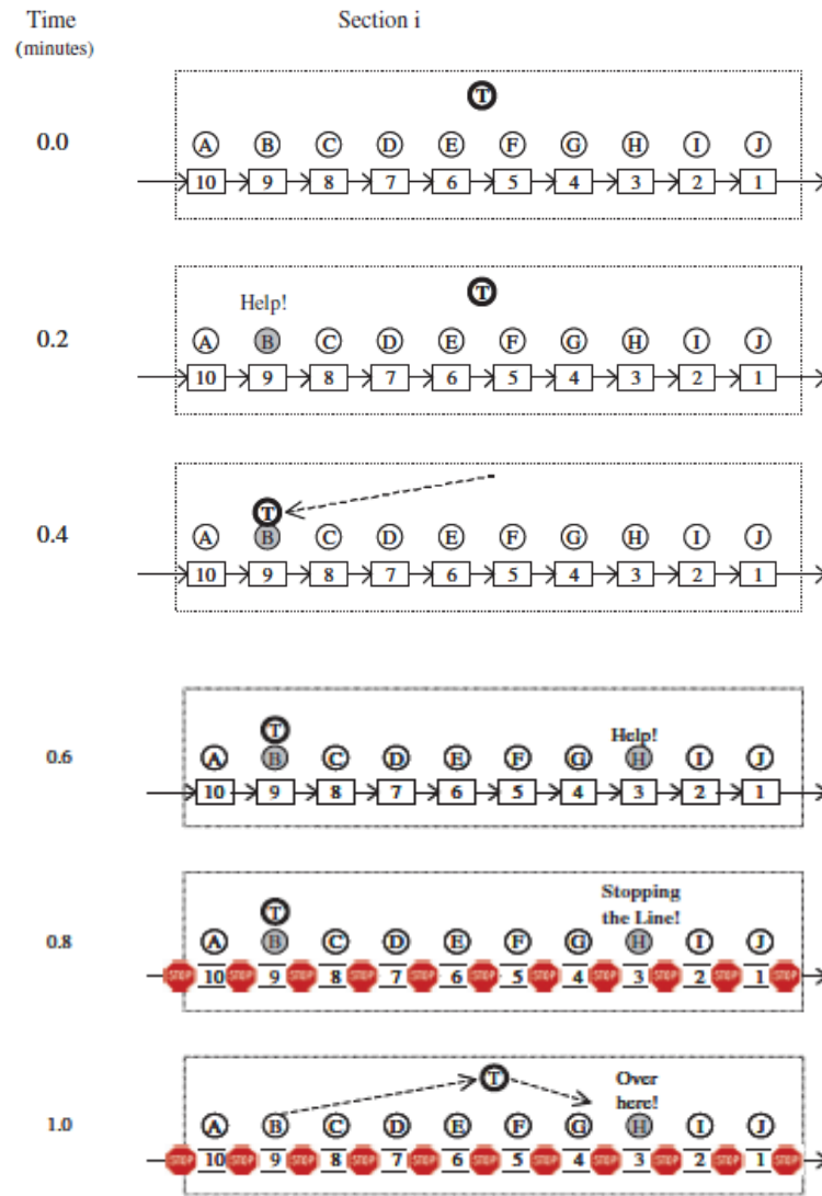
Figure 2.2: Two workers needing help on a section with andon.
