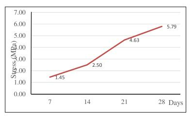
Figure 1: Compressive strength of SYLCAG 1300 kg/m<sup>3</sup>
