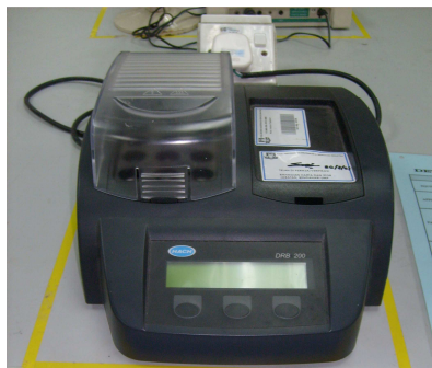
Figure D.1 (a): Digital Reactor Block 200
