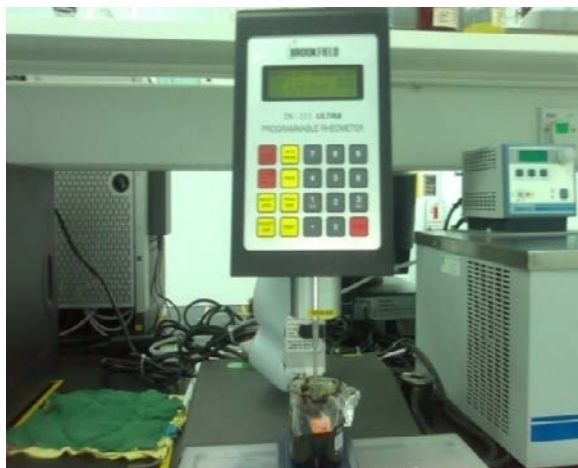
Figure 3.15: Configuration of viscosity analysis using viscometer
