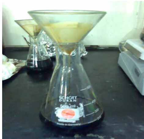
Figure 3.8: Filtration using thin filter paper carried out in the lab
