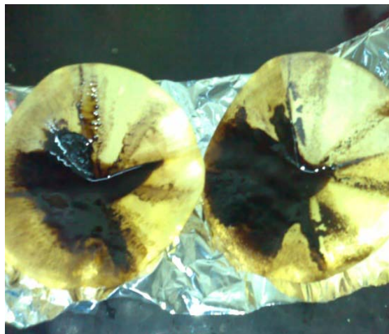
Figure 3.9: Deposition of sludge on filter paper
