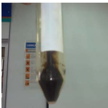
Figure 3.10: Sludge deposition at the bottom of the centrifuge tube
