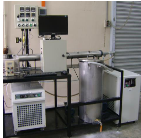
Fig. 1. (a) Schematic Diagram of Force Convection; (b) Force Convection Experimental Setup in laboratory
