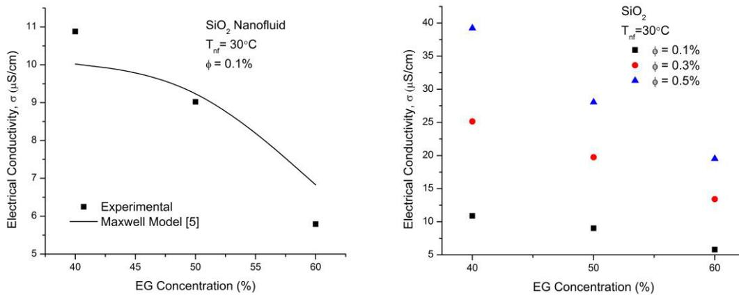
Fig. 3 (a) Comparison of experimental electrical conductivity and Maxwell model; (b) The electrical conductivity of SiO<sub>2</sub> nanofluids with volume concentration of 0.1%, 0.3% and 0.5% at different EG concentration
