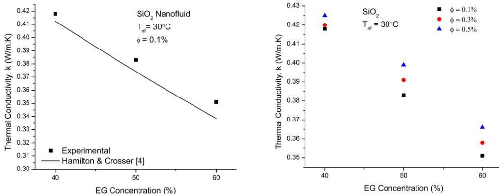
Fig. 1 (a) Comparison of thermal conductivity with Hamilton and Crosser model; (b) Comparison of thermal conductivity in different EG concentration
