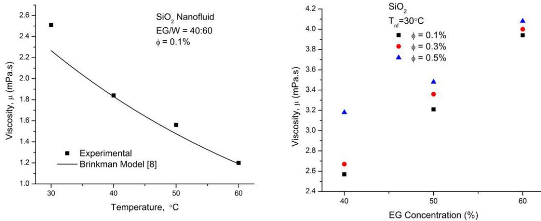
Fig. 2(a) Comparison of experimental viscosity with Brinkman model across the temperature; (b) The Viscosity of SiO<sub>2</sub> nanofluids with volume concentration of 0.1%, 0.3% and 0.5% at different EG concentration
