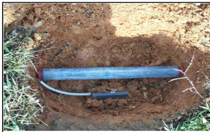
Figure 3.11 Cathodically Protected Uncoated Steel Pipe with Mg
