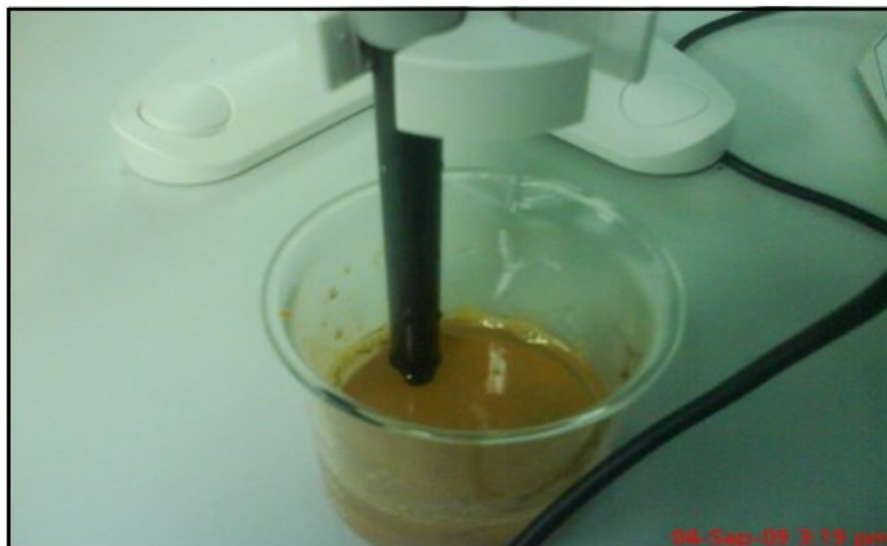
Figure 3.7 Soil Testing Method using pH Meter
