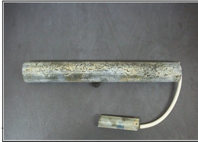
Figure 4.6 cathodically Protected Uncoated Steel pipes with Magnesium Anode
