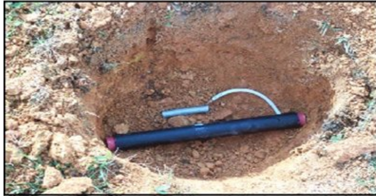
Figure 3.9 Cathodically Protected Coated Steel Pipe with Zn
