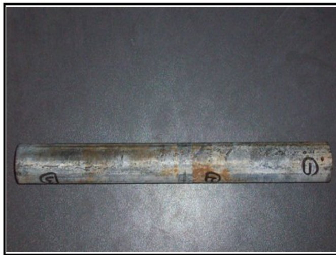
Figure 4.7 Unprotected Steel Pipes
