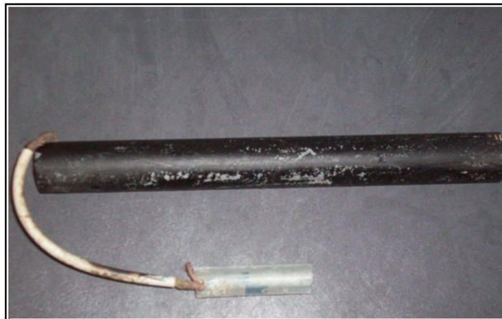
Figure 4.3 Cathodically Protected Coated Steel pipe with Zinc Anode
