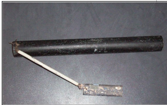
Figure 4.2 Cathodically Protected Coated Steel pipes with Magnesium Anode
