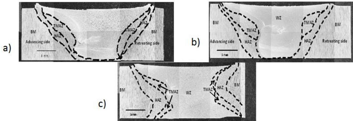
**Figure 3.** Cross section area for FSW joint. a) SP joint, b) NDP joint and c) DSP joint.
