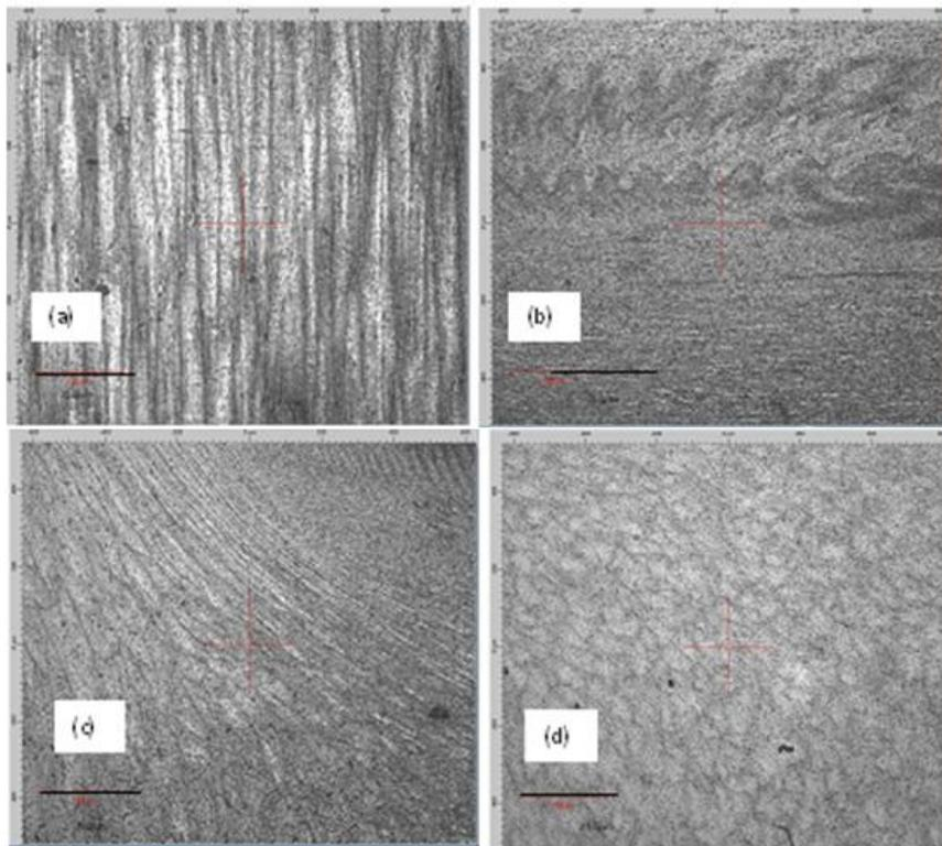
**Figure 4.** Microstructure for SP sample (a) BM, (b) WZ, (c) TMAZ and (d) HAZ.
