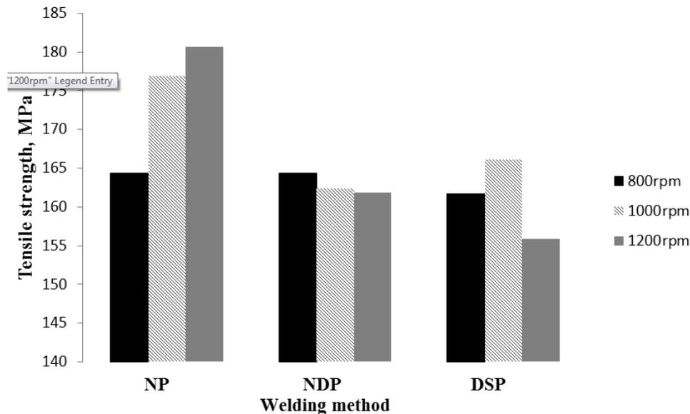
**Figure 8.** Tensile test results for group 1, group 2 and group 3.
