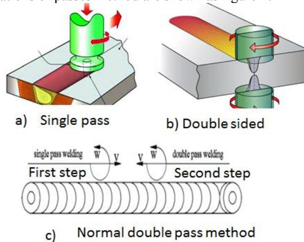
**Figure 1.** Welding passes method. a) Single pass, b) Double sided pass method and c) Normal double pass method [9, 10].
