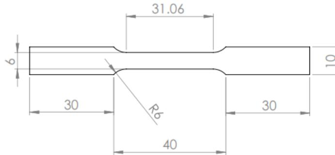
**Figure 2.** Tensile specimen dimensions.
