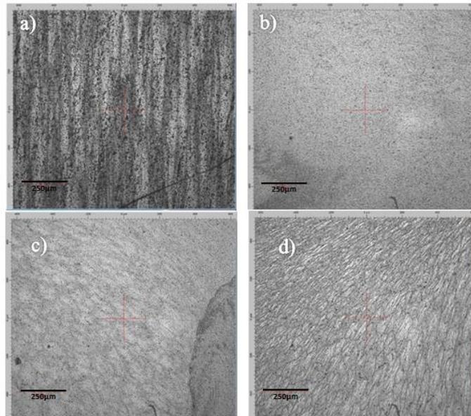
**Figure 5.** Microstructure for NDP sample (a) BM, (b) WZ, (c) TMAZ and (d) HAZ.
