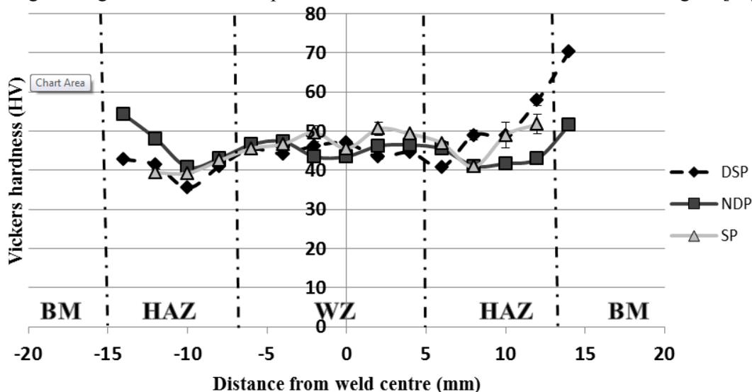
**Figure 7.** Vickers hardness profile for single pass (SP), normal double pass (NDP) and double sided pass (DSP) method.
