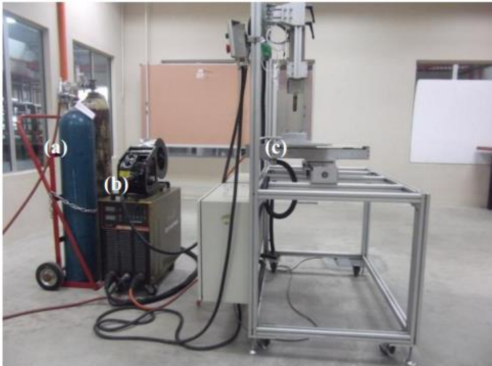
Figure 1. The welding machine and its apparatus used in experiments (a) welding gas, (b) wire feeder and (c) welding table.
