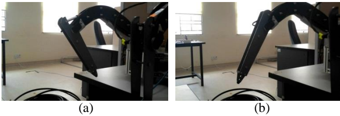
Fig. 16. Joint 3 running procedure, (a) minimum angle position (b) maximum angle position
