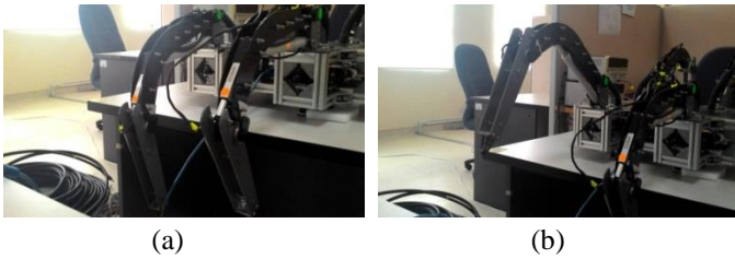
Fig. 15. Joint 2 running procedure, (a) minimum angle position (b) maximum angle position
