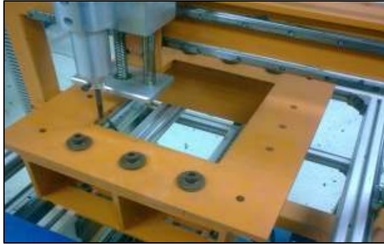
Figure 3.9: Incremental Forming Clamping Area
