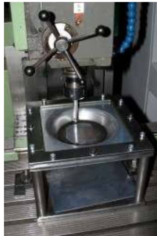
Figure 2.9: NC Milling Machine Configuration Used For Forming A Conical Cup
