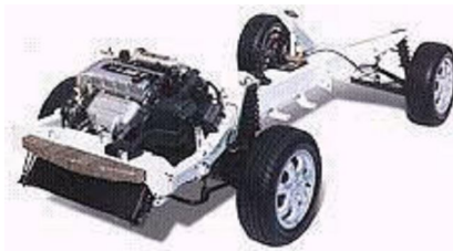
Figure 2.2: The Lotus Elan backbone chassis (Wan, 1998-2000)
