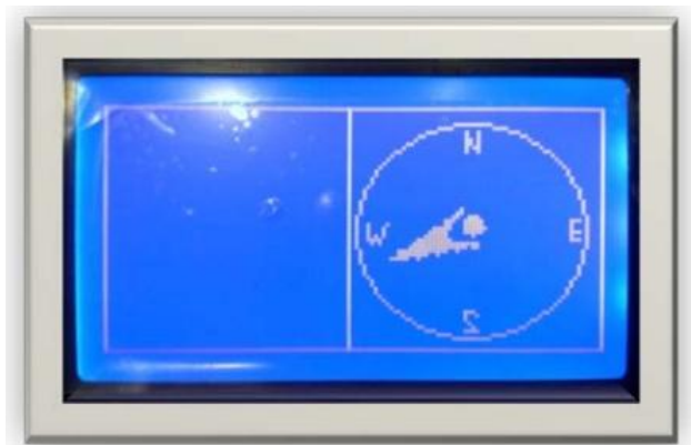
Fig. 9 Screenshot of GLCD showing directional position of Remote Unit with respect to North
