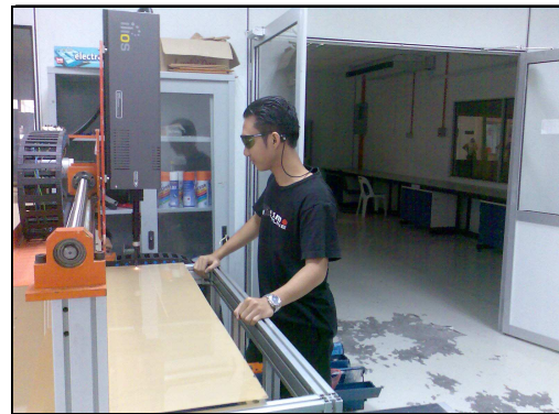
Fig 4.20 Cutting material using automated laser cutter
