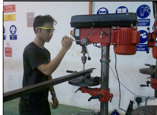
Fig 4.22 Make fastener mating point using drilling machine
