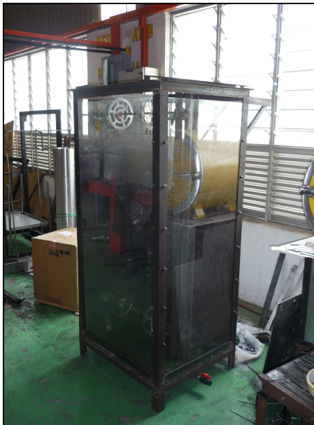
Fig 4.30 Water tank is covered with acrylic to allow operational observation
