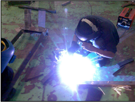
Fig 4.23 Mating parts using arc welding
