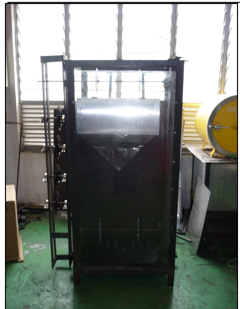
Fig 4.31 Water tank with one set air trap assembled
