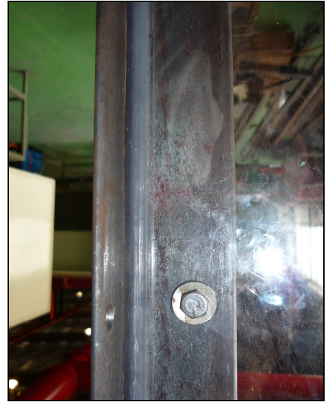
Fig 4.29 Water tank is sealed with silicon to avoid leakage
