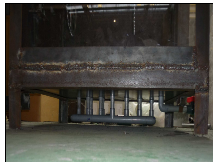
Fig 4.27 Air inlet and water outlet piping system
