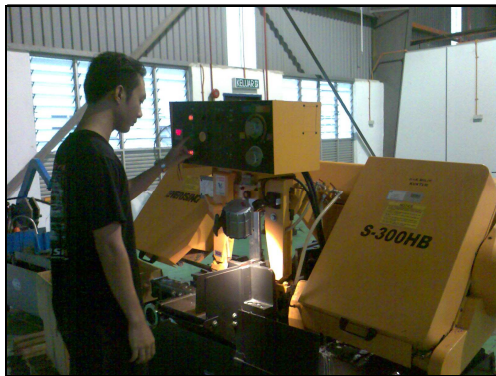
Fig 4.19 Cutting material using automatic band saw machine
