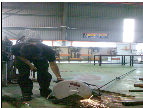
Fig 4.21 Cutting material using disk cutter
