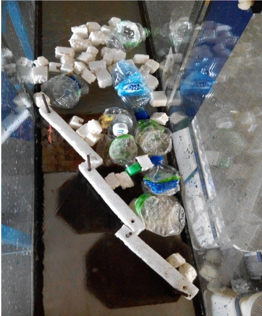
Figure 4.16: Floating debris captured by Styrofoam boom when testing with water level 20mm, all the debris was blocked by the boom.
