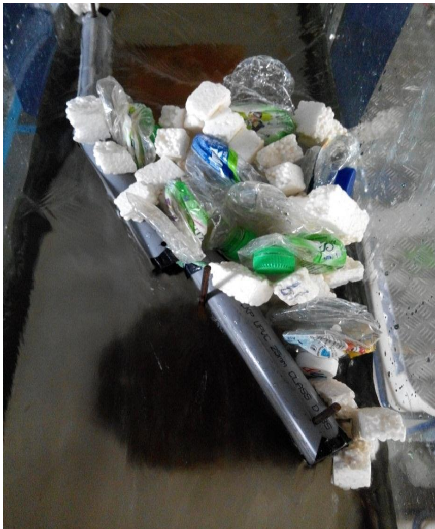
Figure 4.6: Floating debris captured by PVC boom when testing with water level 100mm, half of the debris was blocked by the boom, half has been pass through it.
