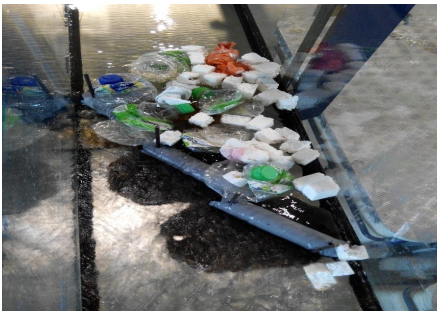
Figure 4.13: Floating debris captured by PVC boom when testing with water level 20mm, all the debris was blocked by the boom.
