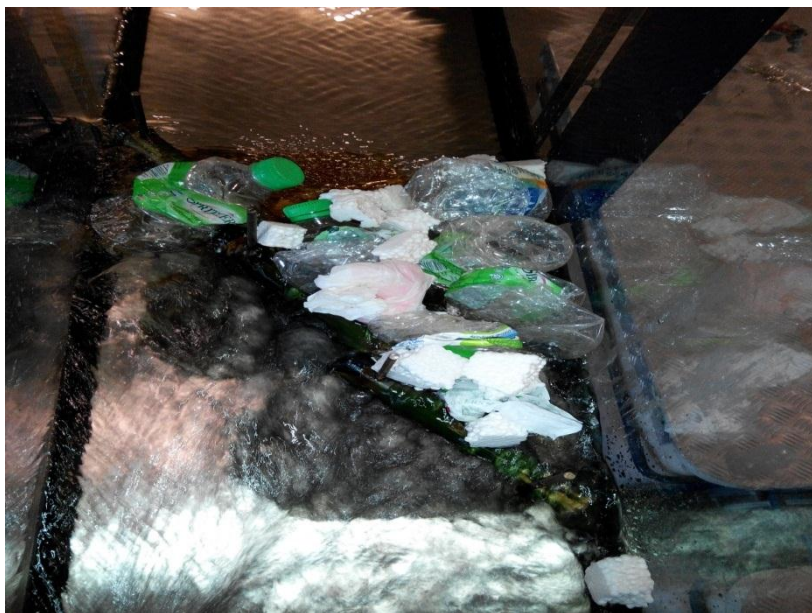
Figure 4.11: Floating debris captured by bamboo boom when testing with water level 60mm, half of the debris was blocked by the boom.
