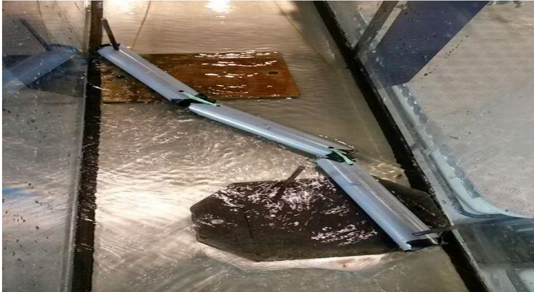
Figure 3.11: Booms with hinged connection are placed in the rectangular open channel to test the effectiveness of the boom.
