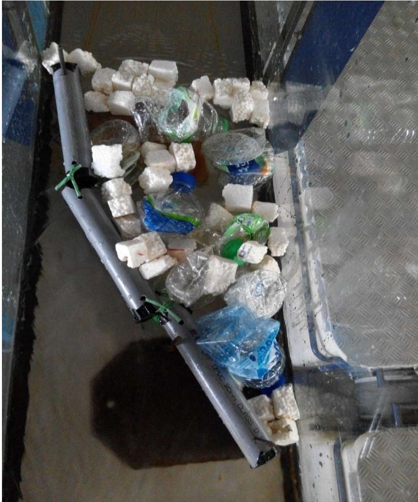
Figure 4.5: Floating debris captured by PVC boom when testing with water level 60mm, the boom was still able to block the debris, some of the debris started to pass through it.
