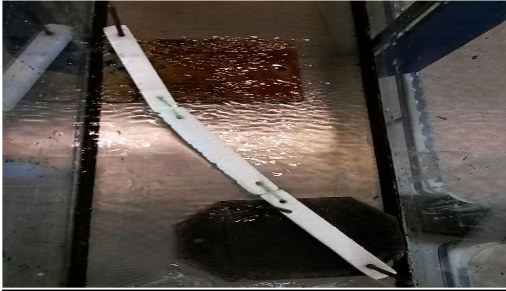
Figure 3.13: Booms with hinged connection are placed in the rectangular open channel to test the effectiveness of the boom .
