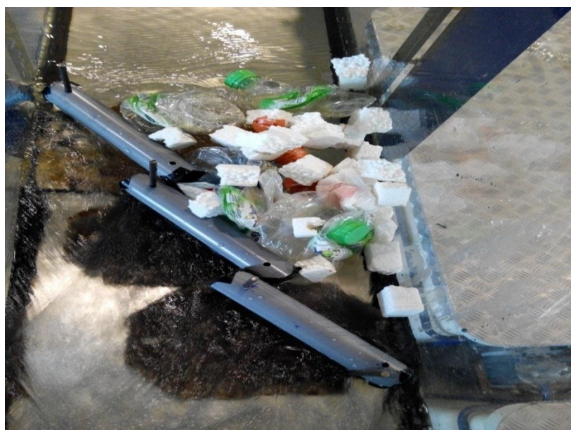
Figure 4.14: Floating debris captured by PVC boom when testing with water level 60mm, some debris started to pass through the boom.
