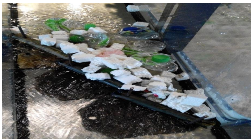
Figure 4.10: Floating debris captured by bamboo boom when testing with water level 20mm, all the debris was blocked by the boom.
