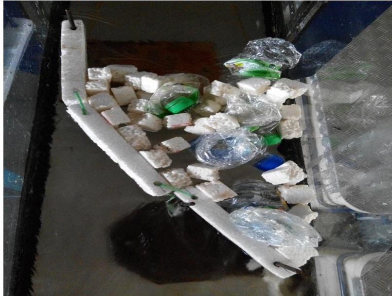
Figure 4.8: Floating debris captured by Styrofoam boom when testing with water level 60mm, all the debris was still able to block by the boom.
