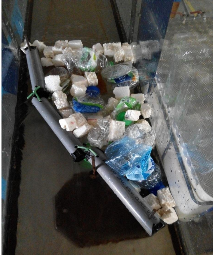
Figure 4.4: Floating debris captured by PVC boom when testing with water level 20mm, all the debris was blocked by the boom.
