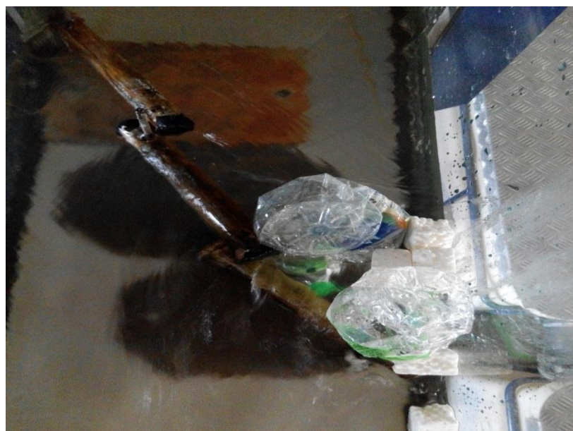
Figure 4.12: Floating debris captured by bamboo boom when testing with water level 100mm, few debris was blocked by the boom.
