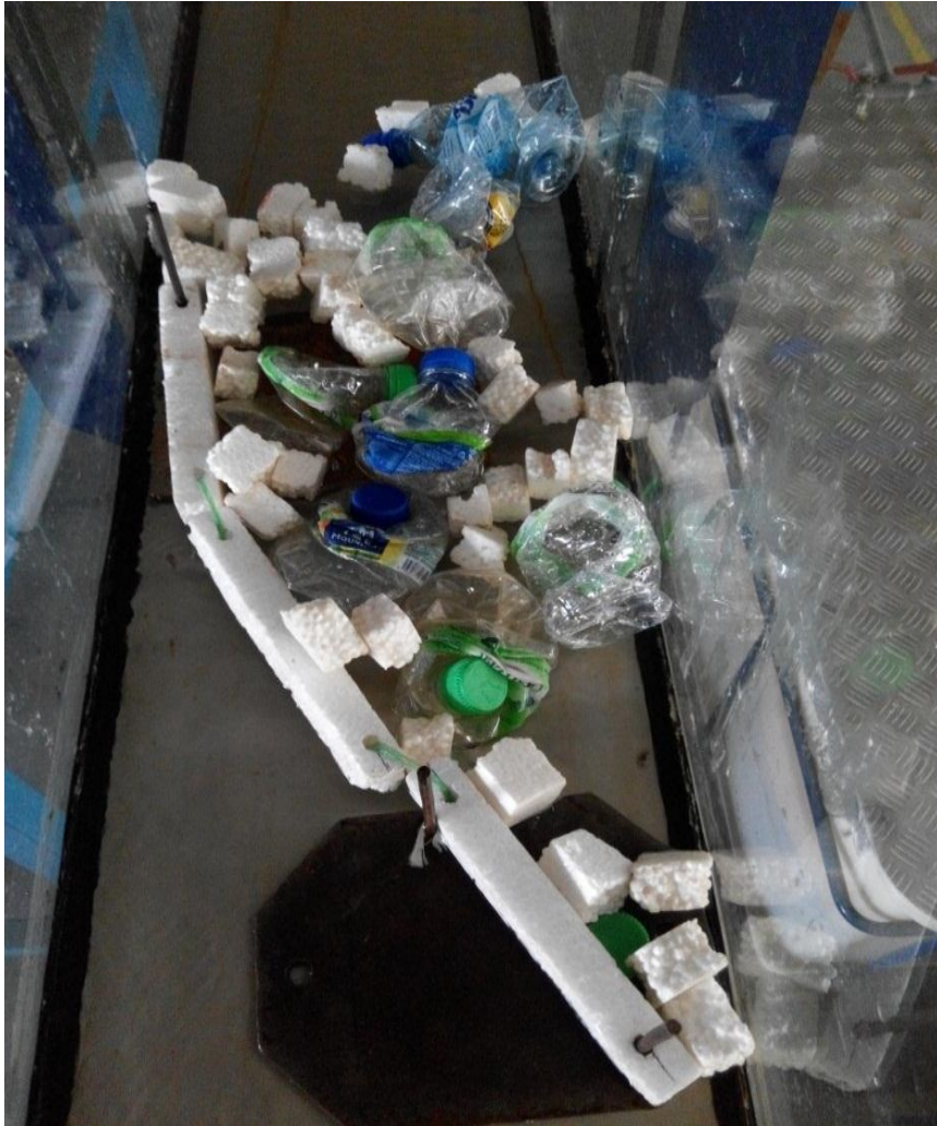
Figure 4.7: Floating debris captured by Styrofoam boom when testing with water level 20mm, all the debris was blocked by the boom.
