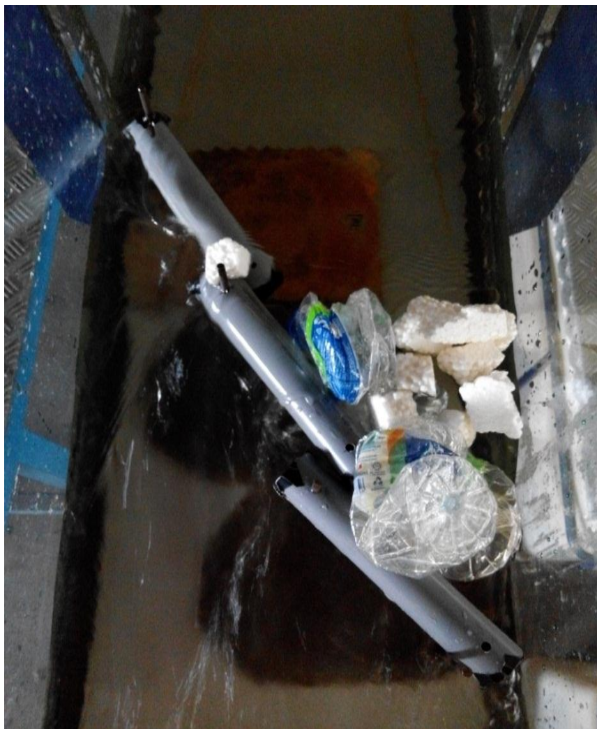
Figure 4.15: Floating debris captured by PVC boom when testing with water level 100mm, some debris stuck at the boom.
