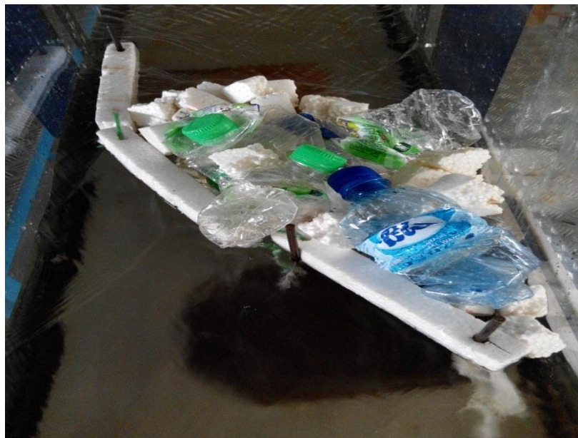
Figure 4.9: Floating debris captured by Styrofoam boom when testing with water level 100mm, \frac{1}{4} of debris has passed through the boom.
