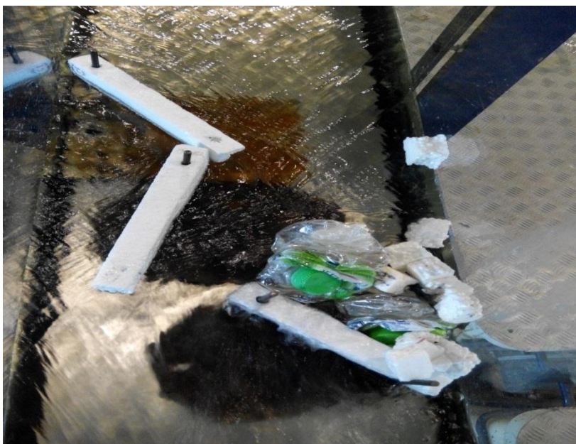
Figure 4.18: Floating debris captured by Styrofoam boom when testing with water level 20mm, all the debris was blocked by the boom.
