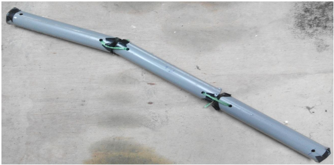
Figure 3.10: Hinged connection was connected by nylon rope between each boom member.
