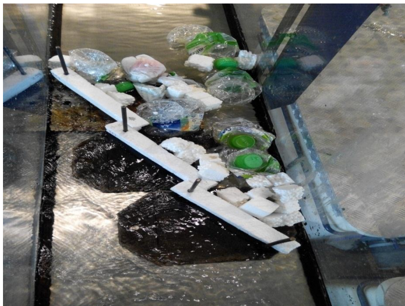
Figure 4.17: Floating debris captured by Styrofoam boom when testing with water level 20mm, all the debris was blocked by the boom.
