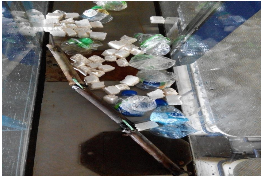
Figure 4.1: Floating debris captured by bamboo boom when testing with water level 20mm, all the debris was blocked by the boom.
