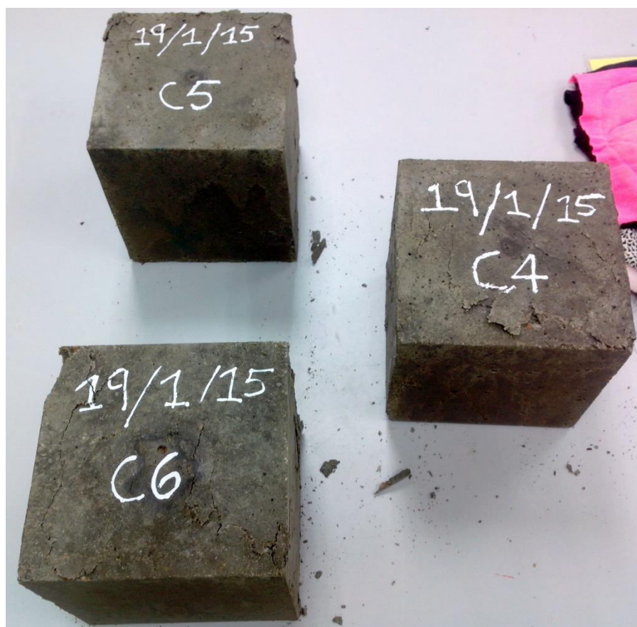
Cube samples after testing at day 7
