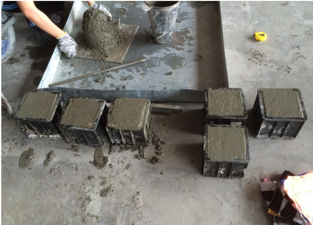
Figure 3.6: Sampling of cubes and slump test
