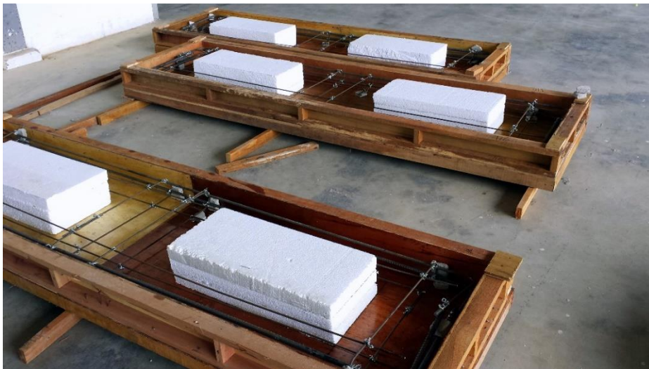
Figure 3.5: Mould of opening
