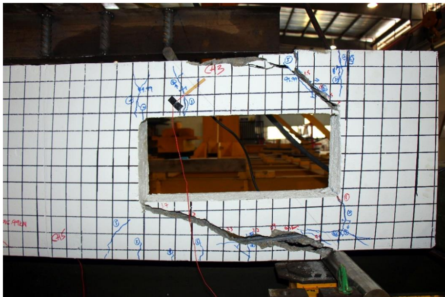
Figure 4.10: Formation of diagonal cracks at the top and bottom chords below and above the openings
