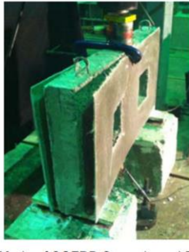
Figure 2.24: Failure mode of SGFRP strengthened beam specimen observed by Ban & Abduljalil
