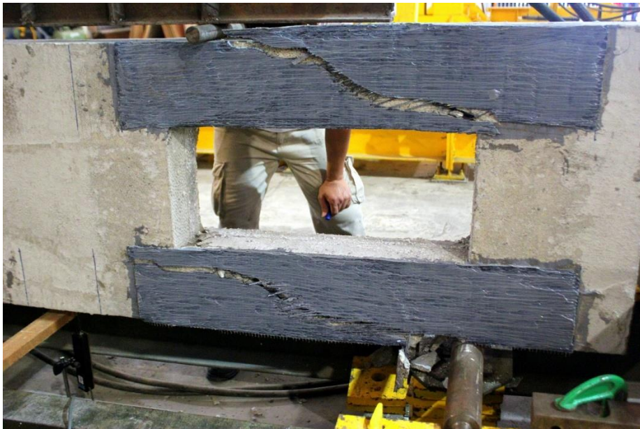
Figure 4.18: CFRP wraps torn at the top and bottom chords below and above the opening
