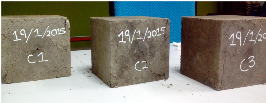
Cube samples after testing at day 3
