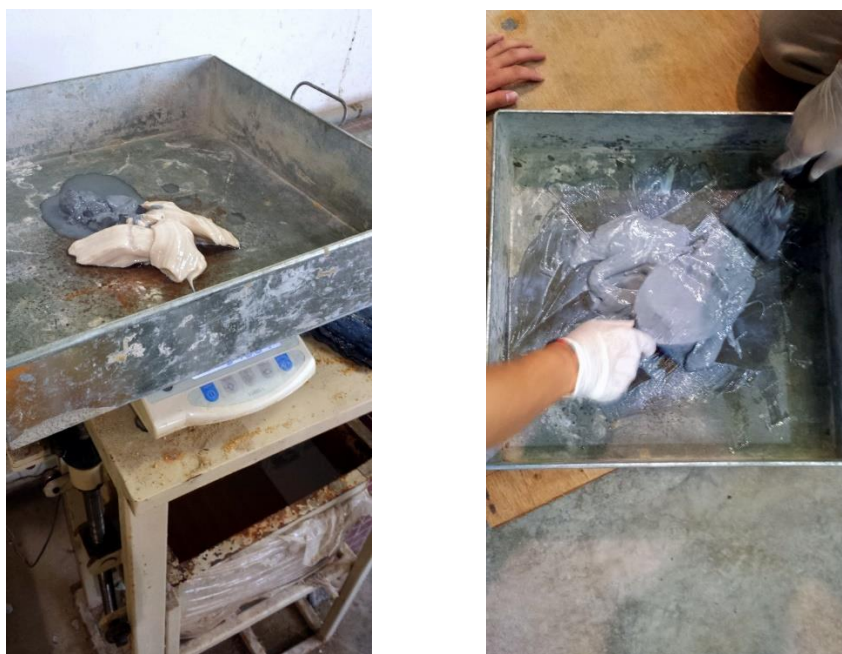
Figure 3.12: Weighing and mixing resin part A and hardener part B with a ratio of 4:1 according to the required weight
