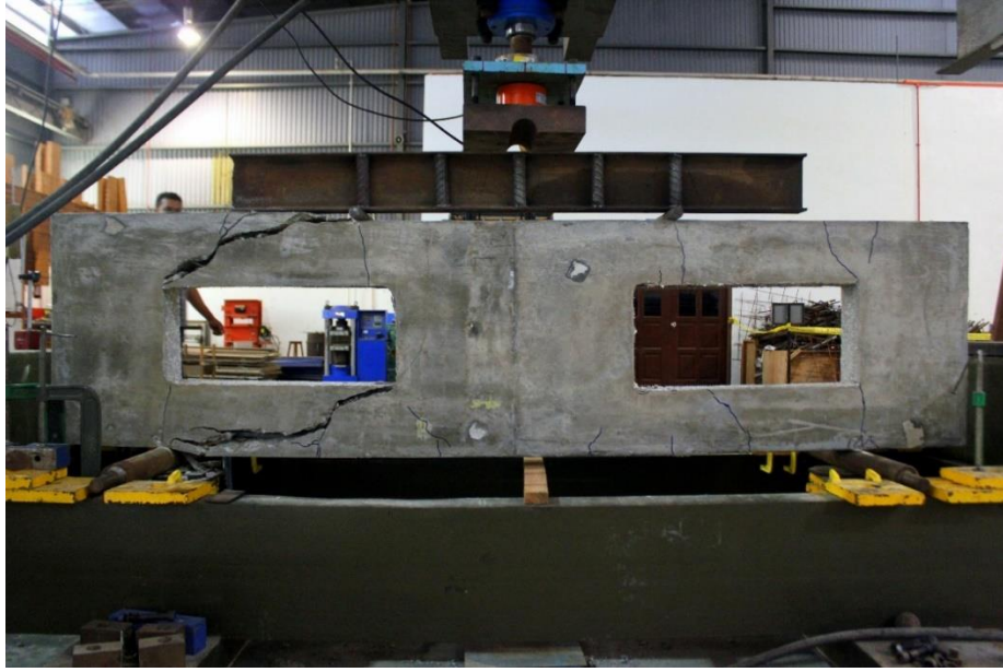
Figure 4.17: Rear view of beam S-BRO-2 after failure
