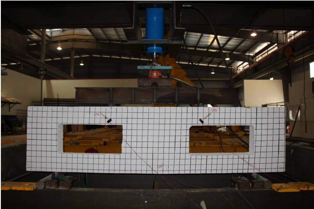
Figure 3.14: Beam testing setup
