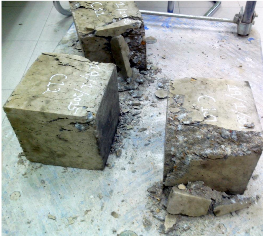
Cube samples after testing at day 28
