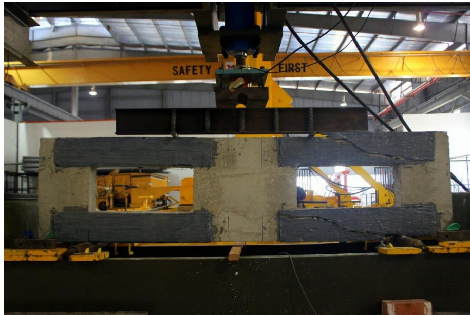
Figure 4.16: Front view of beam S-BRO-2 after failure
