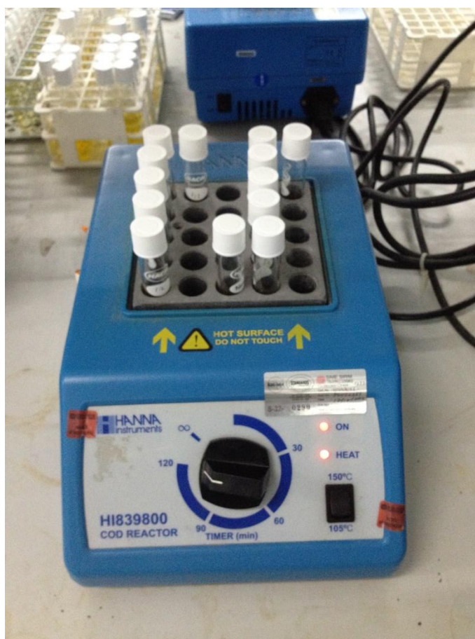
Figure D6: COD Test
