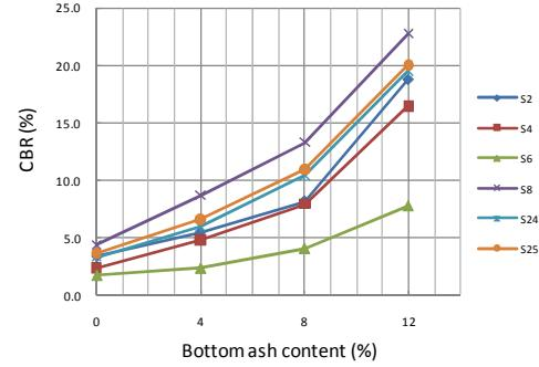
Figure 7. The relationship between bottom ash content and CBR value
