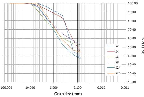
Figure 3. Grain size distribution curves of Kuantan clay
