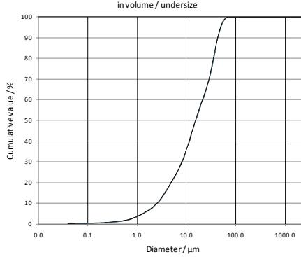
Figure 1. Grain size distribution of fly ash (Kucing, Sarawak source)
