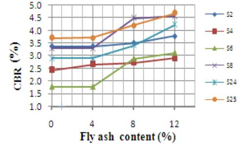
Figure 6. The relationship between fly ash content and CBR value
