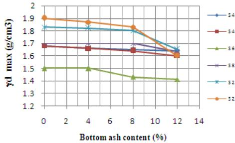
Figure 5. The relationship between bottom ash content and dry unit weight.
