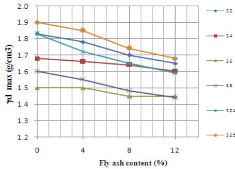
Figure 4. The relationship between fly ash content and dry unit weight.
