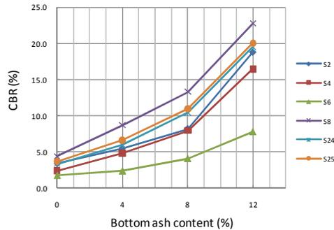
Figure 7. The relationship between bottom ash content and CBR value
