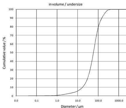
Figure 2. Grain size distribution of bottom ash (Kucing, Sarawak source)
