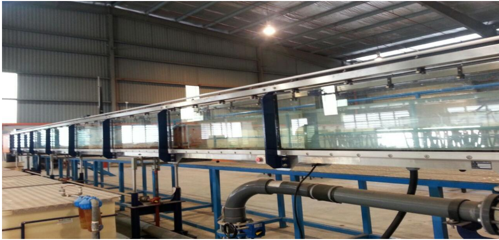
Figure 3.2: Open channel that is located at the Hydraulic and Hydrology Laboratory
