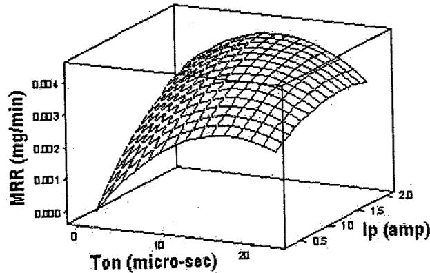
**Figure 4:** Response surface of material removal rate versus pulse-on-time and peak current
