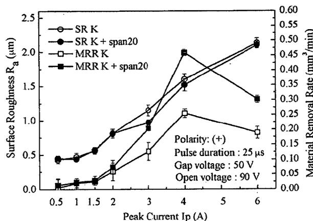
**Figure 1:** Influence of peak current on surface roughness and material removal rate: (SR) Surface roughness, (MRR) Material Removal Rate, and (K) kerosene
