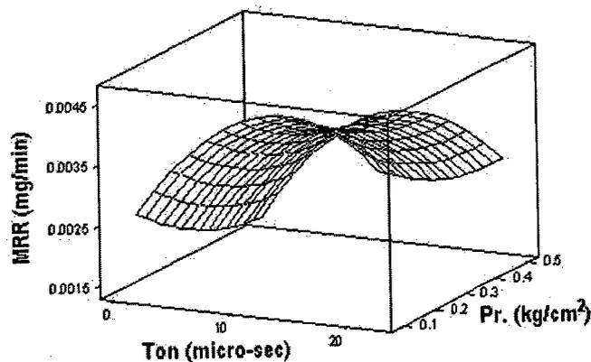
**Figure 5:** Response surface of material removal rate versus pulse-on-time and flushing pressure
