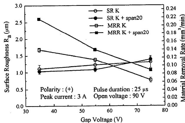
**Figure 2:** Influence of gap voltage on surface roughness and material removal rate: (SR) Surface roughness, (MRR) Material Removal Rate, and (K) kerosene
