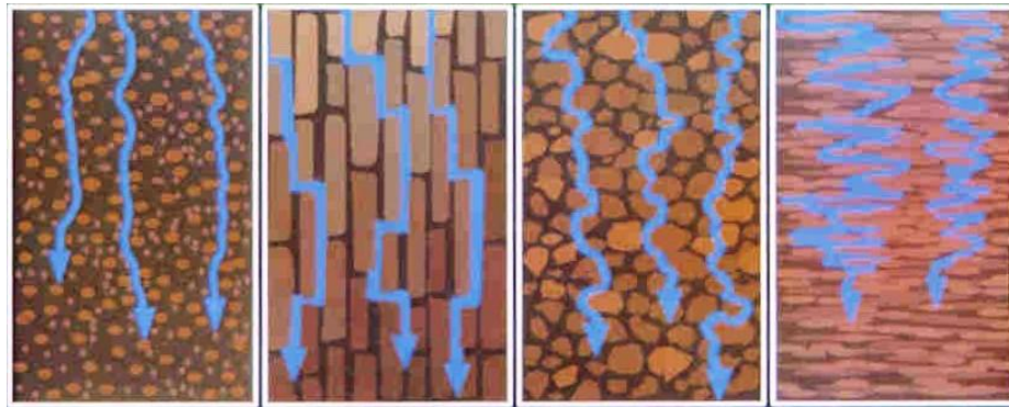
Figure 2.6: Paths of Water Flow through Soils with Granular, Prismatic, Subangular Blocky, and Platy Structure, respectively
