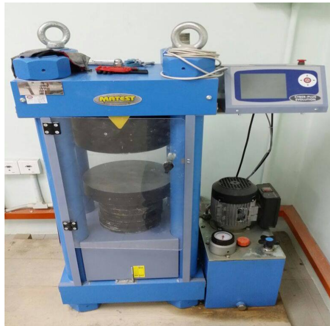
Figure 3.14: Compressive Strength Machine
