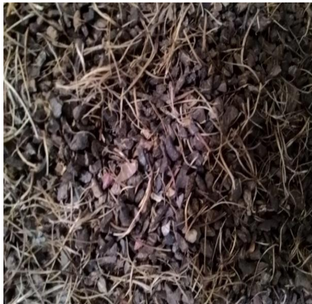
Figure 3.2: Palm Kernel Shell with size between 1.5mm to 2.36mm
