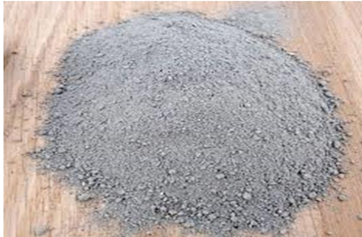
Figure 3.6: Ordinary Portland Cement
