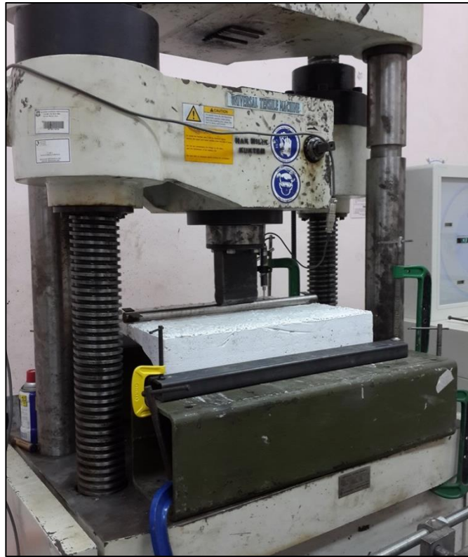
Figure 3.15 : Testing of arch tile setup using Universal Tensile Machine.
