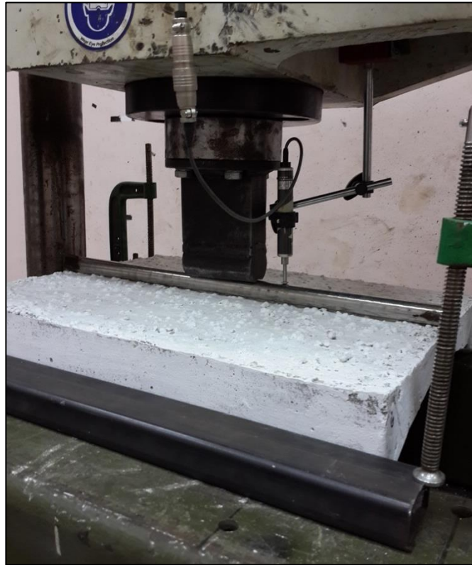
Figure 3.16 : Linear Vertical Displacement Transducer (LVDT) is use to measures displacement
