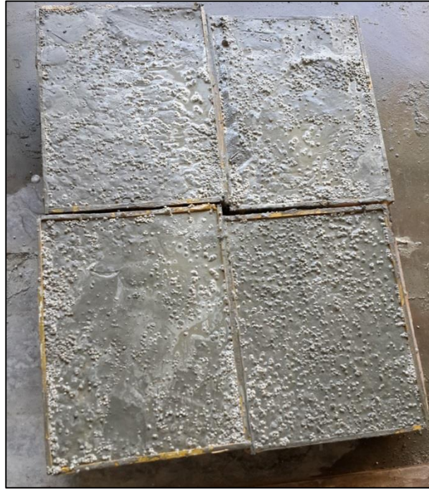
Figure 3.12 : Complete casting of slab.
