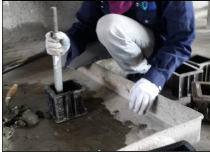
Figure 3.9 : Blowing step for compacted the concrete in cube mold
