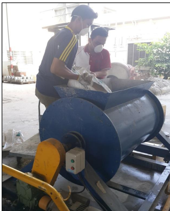
Figure 3.10 : Lightweight concrete mixer of 0.5m 3 capacity used for lightweight concrete mixing.
