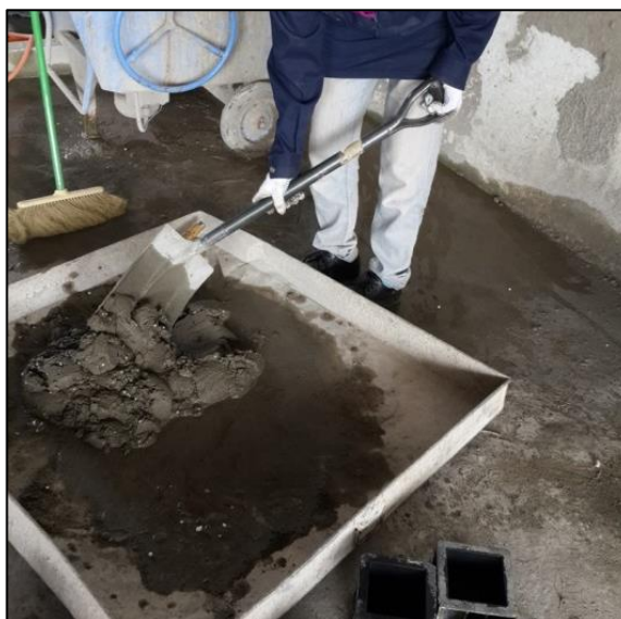
Figure 3.8 : Manual mixing by hand concrete mixing for trial mix.
