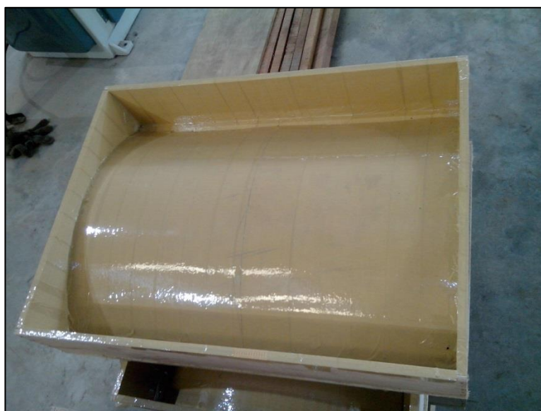
Figure 3.6 : Completed arch tile formwork
