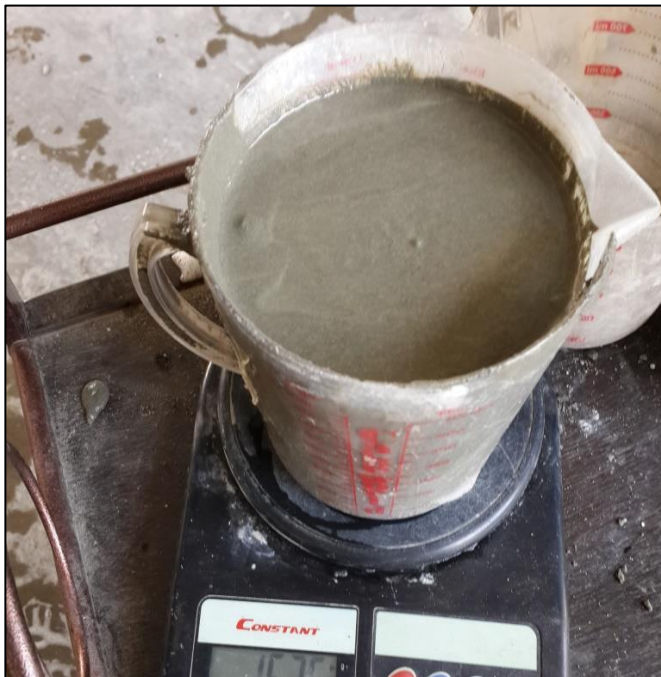
Figure 3.18 : Weigh the fresh concrete.
