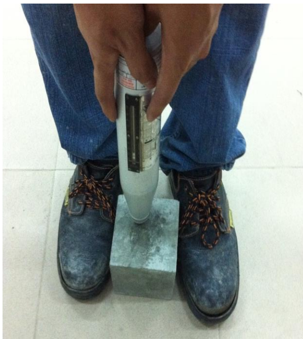
Figure 3.12: Rebound Hammer Test
