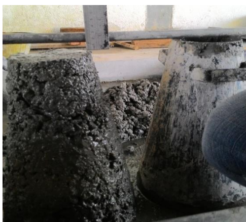
Figure 4.2: Slump result of NA
