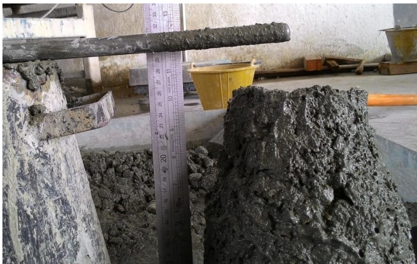
Figure 4.3: Slump result of PA 2
