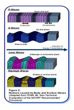
Figure 2.1: Motion of Body and Surface waves
