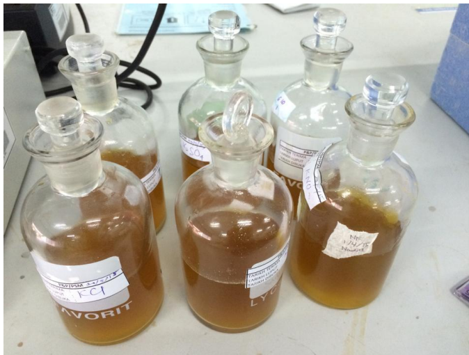
Figure 3.4 Soil extracted following the soil survey standard test method : organic carbon
