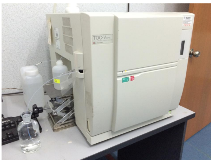
Figure 3.6 Total Organic Carbon (TOC) Analyser used in this study
