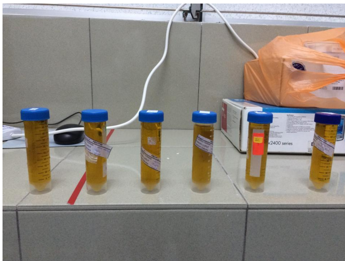
Figure 3.5 Extracted soils in 50 mL centrifuge tubes
